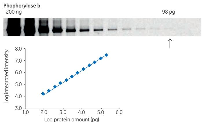
**Fig 7.** Evaluation of linearity, dynamic range, and limit of detection for fluorescence detection with Amersham Imager 600. A two-fold dilution series of phosphorylase b pre-labeled with Cy5 shows a dynamic range of 3.3 orders of magnitude.
