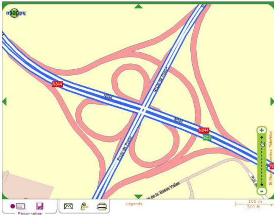
Fig. 5. Mappy (TeleAtlas data) map rendering of Cheviré south interchange. One-way roads are represented by one poly-line, which makes two poly-lines for highways (in blue), and one for exits (in orange). Shape points are visible in curves. Multiple lane exits are simplified. Lanes separation due to bridge piles at highways crossing is not represented.
