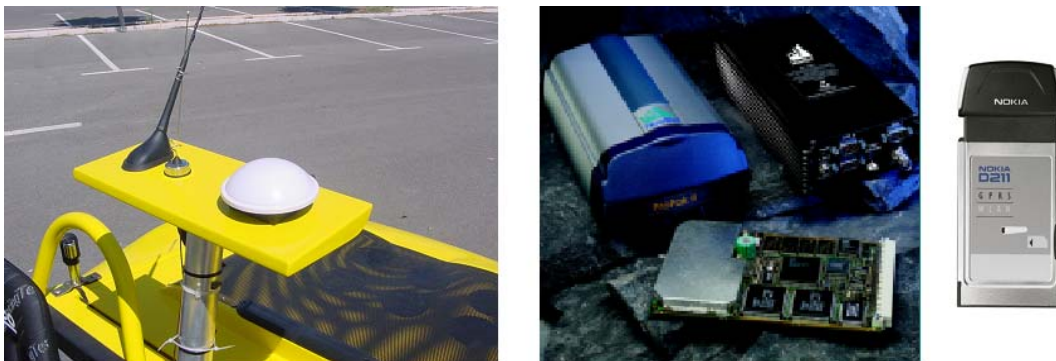
Figure 3.- (a)Vehicle Comarth S1-50. (b) GNSS sensor, Novatel. (c) GPRS/WLAN board
