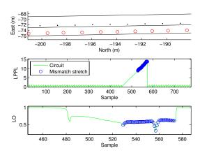
Fig. 5. (Top) A stretch of estimated vehicle trajectory during a mismatch: road lanes (solid black), ground truth (black ·), filter positions (red o). (Middle) LPPL values along a stretch of the circuit (solid green) and during the period of mismatch (blue o). (Bottom)  $\mu$ LO values along a stretch of the circuit (solid green) and during the period of mismatch (blue o).
