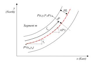
Fig. 2. Cartesian x, y and Frenet  $l^m, d^m$  coordinates for a point P, position of a vehicle driving segment m with a given half lane width HL. Initial angle of the segment  $\tau_0$ , and angle at any Frenet abscissa  $\tau(l_m)$ .
