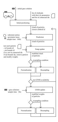
Fig. 3. Flowchart of the single positioning and map-matching fusion process.
