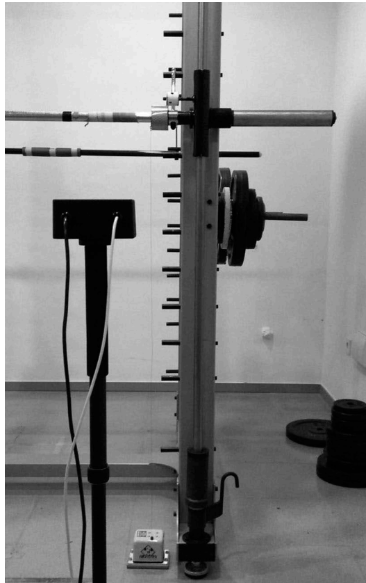
Figure 1. Installation of Velowin and T-Force devices on Smith machine bar.
